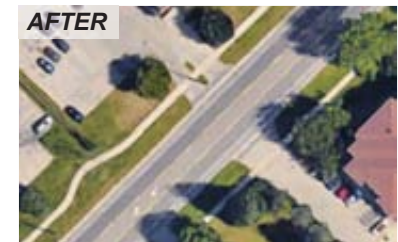
Road diet on College Avenue West in Guelph reduced four travel lanes to two plus a centre turn lane, and made space for a bike lane.
