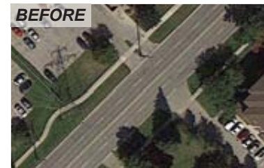
Road diet on College Avenue West in Guelph reduced four travel lanes to two plus a centre turn lane, and made space for a bike lane.
