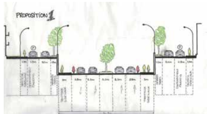
Street cross-sectional view. Design proposal for an underpass on Girouard Avenue.
